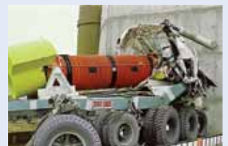
A flatbed semi-trailer carrying a 22-ton Type B Package on it, after being crashed into a 690-ton concrete block at 60 mph.
